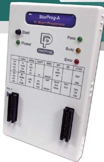
StarProg-A supports MCU, CPLD, SPI NOR Flash, SPI NAND Flash, and EEPROM on board programming (ICP/ISP). It is optimized for the integration of automated machines and can be easily used in development and mass production.
